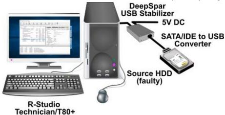
If any drive issue occurs, **USB Stabilizer** handles this issue preventing the system from freezes, crashes, or disconnecting the drive. Such handling may include various drive resets or even drive repower without system loosing the device.
