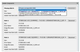
You may immediately switch to the mdadm RAID configuration that **R-Studio** believes most probable by clicking the **Reassemble** button.
