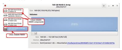
**R-Studio for Linux** detects components from mdadm RAIDs and creates those RAIDs automatically. At the same time, **R-Studio for Linux** gives access to the components of those RAIDs (hard drives and images).
